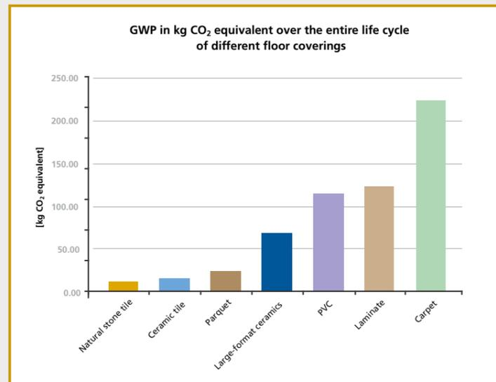
When investigating coverings used for the highest performance floors, it was found that equivalence values for natural stone slabs are lower in all impact categories compared with terrazzo tiles. For example, the GWP of a natural stone slab is about 27% lower than that of a terrazzo tile and about 74% less than that of large-format ceramics.
